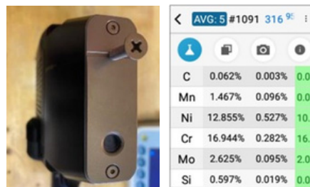
Figure 4 SciAps Z-902 Carbon analysis of 1/8" wire, 316L material
