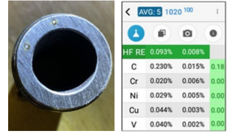
Figure 3 SciAps Z-902 Carbon analysis of 1" s/160 A106 pipe nipple for HF Alkylation service
