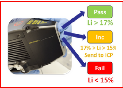
Figure 5: Screening program for lithium carbonate
