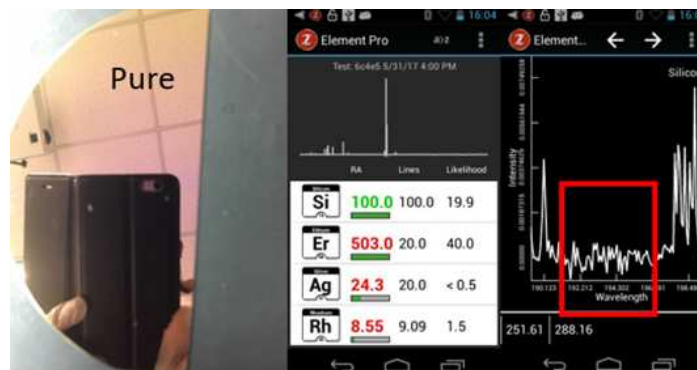
Figure 2: Surface analysis using Element Pro of a clean surface with no carbon contamination
