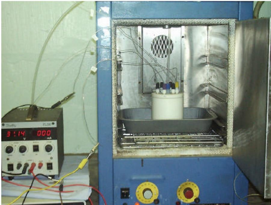
**Figure 3.** PTFE cell fitted with a PTFE condenser for ambient-pressure electrochemical studies.
